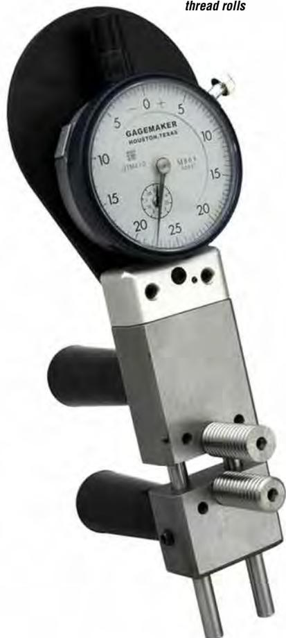
The SPG-6000 line of thread inspection gages measures internal thread diameters smaller than 1.500". The SPG-6000 can be equipped with either thread rolls or contact points. Contact points are used to measure pitch diameter, while thread rolls are used in measuring functional size. **Contact points, contact point arms, software, and thread rolls sold separately.**
